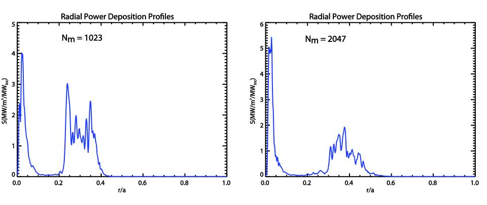
Broadening of the LH power deposition profile is consistent with adding higher k<sub>//</sub> components to the spectral solution in TorLH that correspond to higher m. Parallel electric field of LH wave starts to exhibit features of multiple reflections and weak single pass absorption as N<sub>m</sub> is increased
