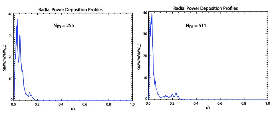
Broadening of the LH power deposition profile is consistent with adding higher k<sub>//</sub> components to the spectral solution in TorLH that correspond to higher m.
