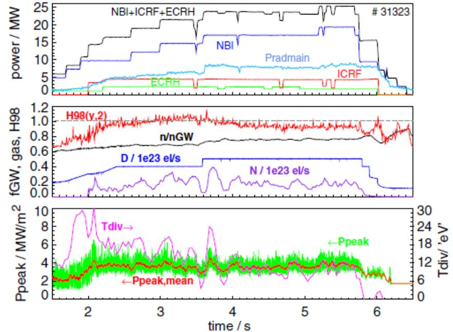
$(P_{\text{sep}}/R)_{\text{max}} = 10 \text{ MWm}^{-1}$  (cf.  $\sim 15 \text{ MWm}^{-1}$  for ITER)
