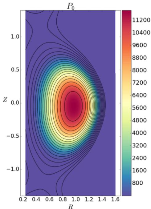
Pressure contours with poloidal flux contour lines superimposed.
