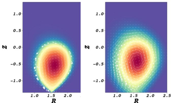
Contours of  $T$  with  $J$  vectors overlaid at  $t = 1410$  with Dirichlet (left) and insulating (right).
