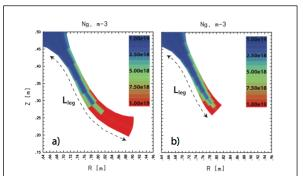
Fig. 1 – Distribution of neutral gas density in a longer (a) and shorter (b) divertor leg shows steady-state location of the detachment front. Regardless of the leg length, the detachment front location is similar for same exhaust power.
