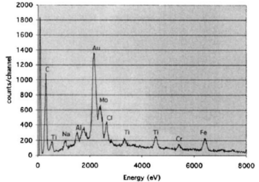
Carbon, steel and titanium particle collected from the LHD coil armor (Sharpe et al., [J. Nucl. Mater, 2003](#))
