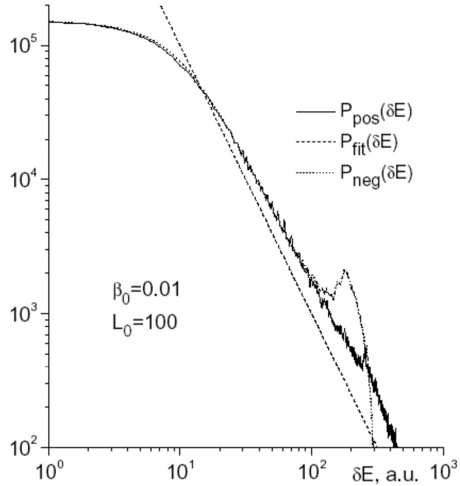
PDF of dust energy gain for “zig-zag” surface,  $P_{\text{fit}}(\delta E) \propto \delta E^{-2}$
