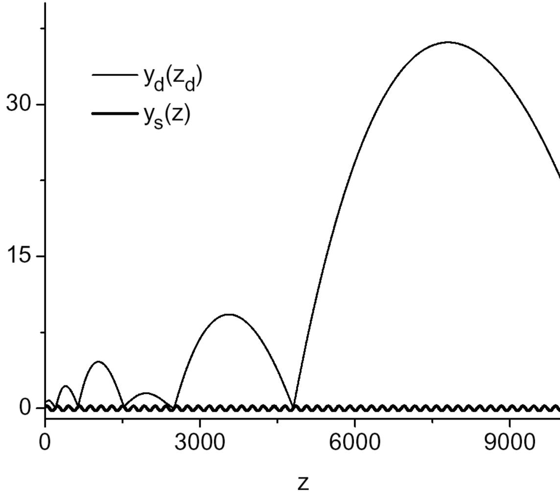
Flights of dust particle over corrugated surface
