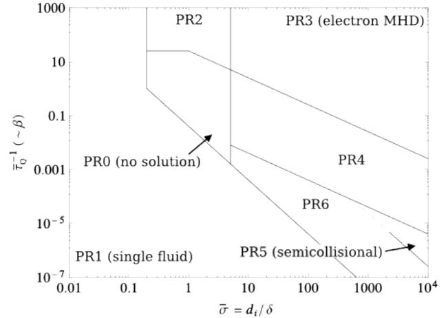
Figure 1: Drift-tearing mode dispersion relation solutions in normalized  $\beta - d_i$  parameter space.
