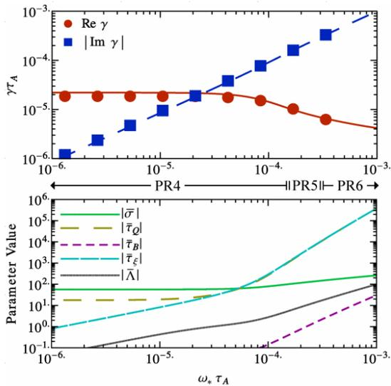
Figure 2: An example drift verification with a comparison of the dispersion relation for the analytics (lines) and NIMROD computations (discrete points).
