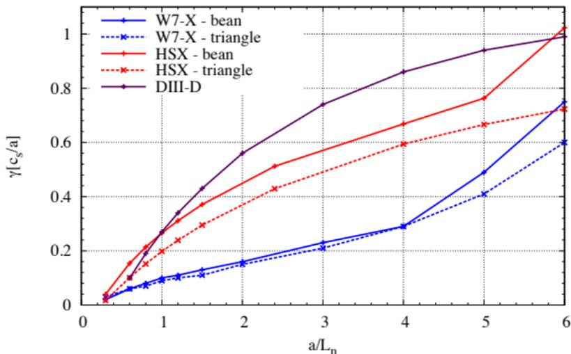
Highest TEM growth rates  $\gamma$  at density gradients  $a/L_n$  with  $a =$  minor radius including DIII-D data for comparison
