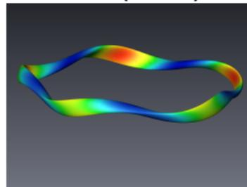
Magnetic field strength  $|\mathbf{B}|$  on the flux surface of  $r/a = 0.5$
