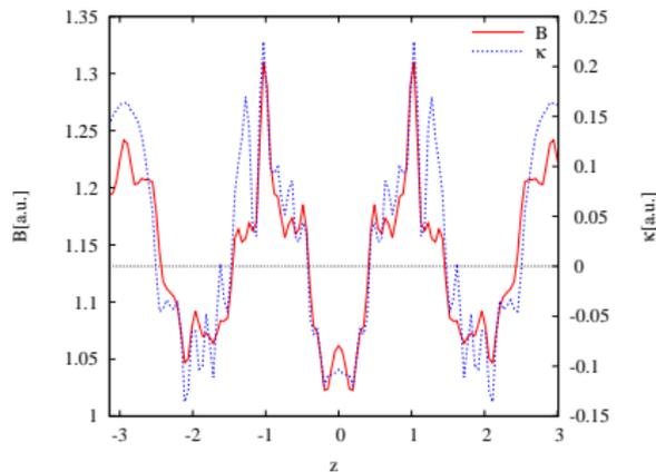
Magnetic field strength  $B$  and curvature  $\kappa$  along a magnetic field line.
