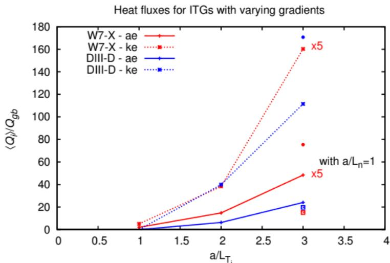
Ion temperature gradient modes with pure ion temperature gradient, with adiabatic (ae) and kinetic (ke) electrons in the DIII-D tokamak and W7-X.
