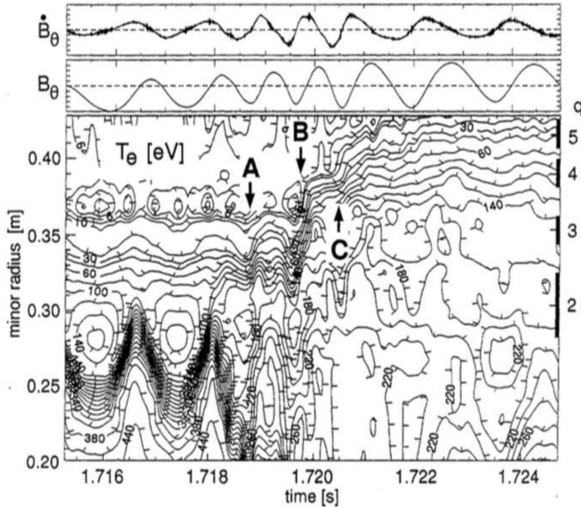
FIG. 4. A minor disruption ( $q_{95} = 6$ ) leads to partial flattening of the  $T_e$  profile and reheating around resonant surfaces, first (A) at  $q = 2$ , then (B) at  $q = 3$  and finally (C) around  $q = 4$ . No mode locking is observed. Mirnov oscillations ( $B_\theta$  measured near the ECE antenna position) appear accelerated during this sequence.
