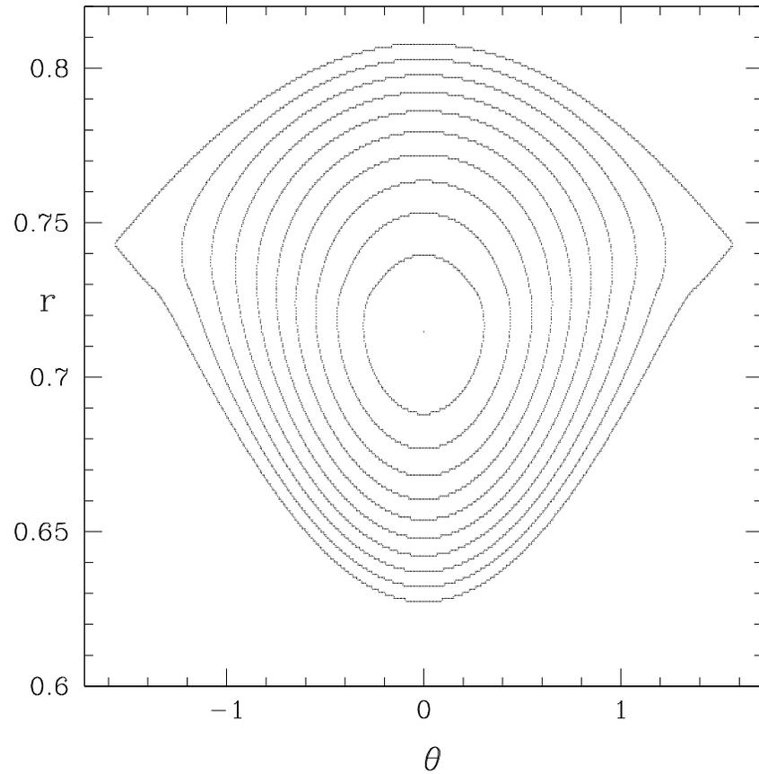
Magnetic islands including the effect of current flattening. The small island has amplitude  $\alpha = 10^{-4}$ , and width  $w = .05$ ,  $A = .26$ . The amplitude of the large island is  $\alpha = 1.5 \times 10^{-3}$ , with width  $w = 0.18$ , and asymmetry  $A = .78$ . Profile parameters are those of the disruption test case with  $f_F = 1$ .
