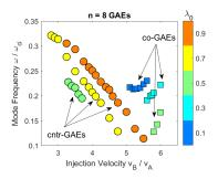
EP-GAE frequency dependence on  $v_0/v_A$ . Color denotes the central pitch  $\lambda_0 = \mu B_0/\mathcal{E}$  of the beam distribution used in each simulation. On-axis  $f_{ci} = 2.4$  MHz.
