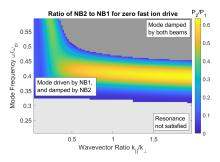
Theoretical predictions of fractional power necessary in off-axis beam (NB2) to stabilize cntr-GAEs driven by on-axis beam (NB1) in NSTX-U
