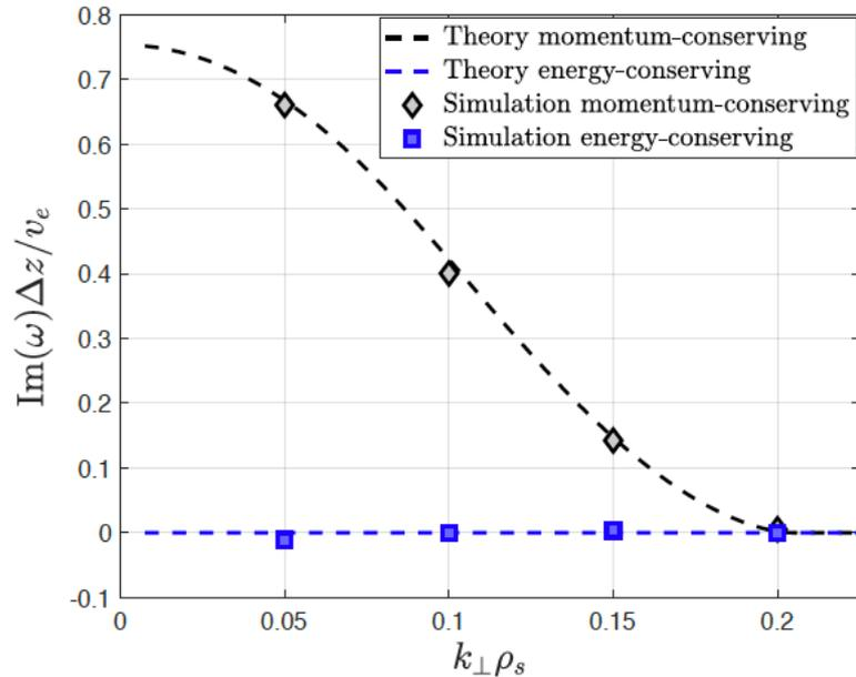
Comparisons of measured growth rates from simulations to growth rates predicted from the numerical dispersion relations.
