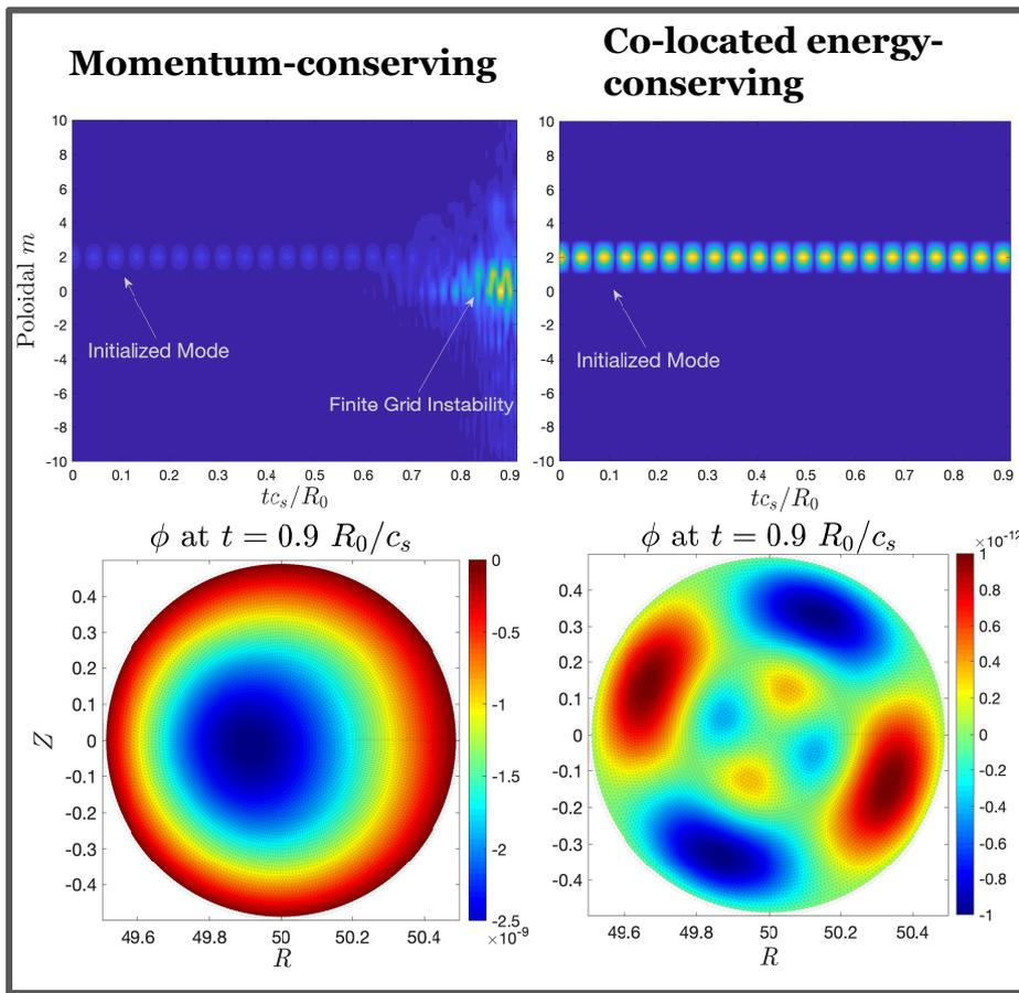
**Figure:** Shear Alfvén waves are excited from an initial perturbation in XGC. With the momentum-conserving scheme (left), the finite-grid instability, characterized by long wavelengths in the poloidal plane, quickly develops. The co-located energy-conserving scheme (right) allows for clean, numerically stable simulations.
